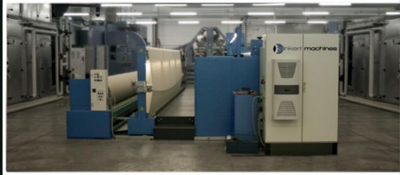
The **MALIVLIES** machine is a high-performance stitch-bonding machine for the mechanical bonding of fed fibrous webs by means of seam-like or surface stitch-bonding.
